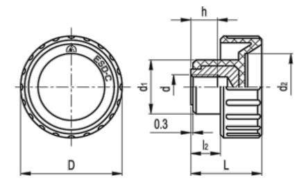
$\begin{array}{lll} D & = 20 \\ d1 & = 11.5 \\ d2 & = 11 \\ d \ 6H & = M5 \\ h & = 6 \\ L & = 16 \\ l2 & = 6 \\ Weight \ (g) = 6 \end{array}$
